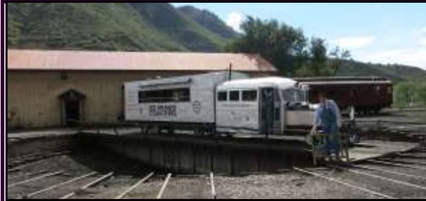
At the end of each day in Durango, No. 5 was driven onto the turntable and pulled into the museum area of the roundhouse.
