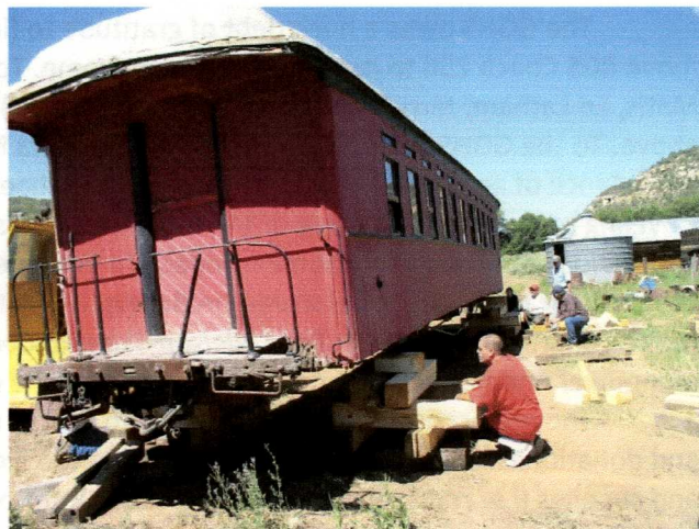
Above left – The coach is loaded and readied for the 3-mile trip to the site where it will be restored. Above right – it is being placed on wooden timber cribbing at Truelsen's mill where it will stay for most of the restoration project.
